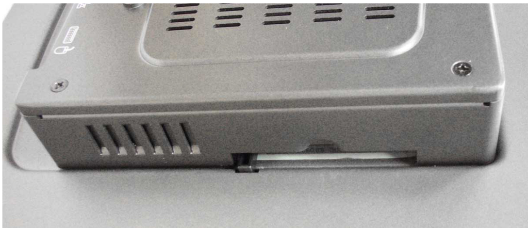
Figure 2.2 Install CFast Memory Card
